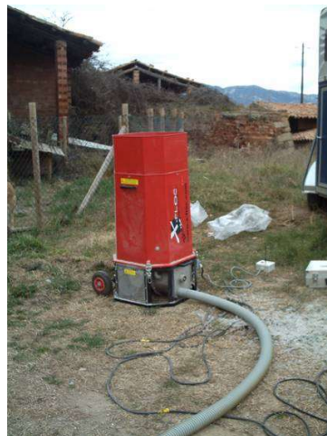
Cellulose projected: 0,040 W/m·K (newspaper, 10% Borax for fire resistance and as fungicide)
