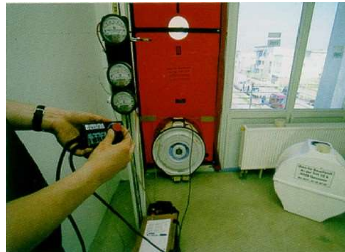
Infiltration control by “Blower-Door-Test”.
