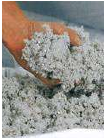
Cellulose projected: 0,040 W/m·K (newspaper, 10% Borax for fire resistance and as fungicide)
